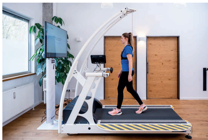
Figure 3. Complete hardware setup recommended by h/p/cosmos (h/p/cosmos treadmill, VAST.Rehab software displayed by and TV, camera)
