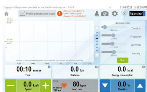
UserTerminal MCU6 featuring a quick generator module for fast and easy perturbation setup and several tests (e.g. Stroop test)
