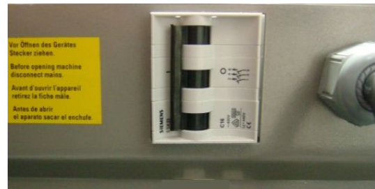
Expulsion fuse, device fuse 3-pole C16A
