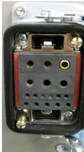
cos100710 socket in UserTerminal for inverter, drive and elevation motor
