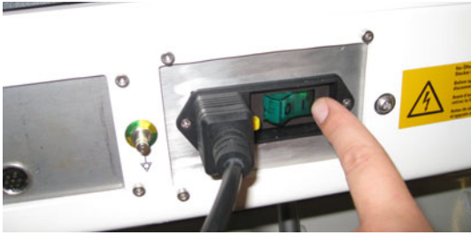
Device protection switch / thermal protectet 16A, ON-OFF switch
