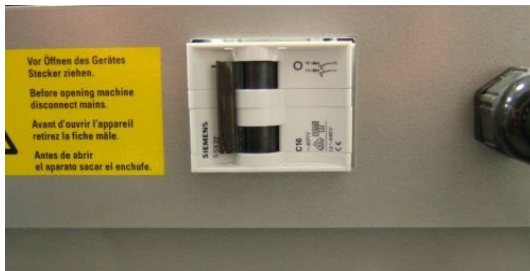
Expulsion fuse/ON-OFF button 2-pole C16A
