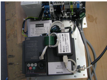
Opto coupler board [cos100601] (only with digital RS485 inverter)
